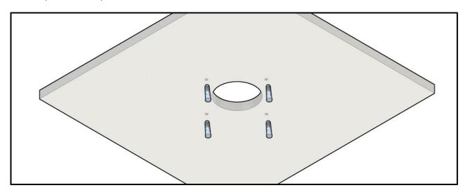
4. Reposition the Base and attach it to the surface using supplied screws.
