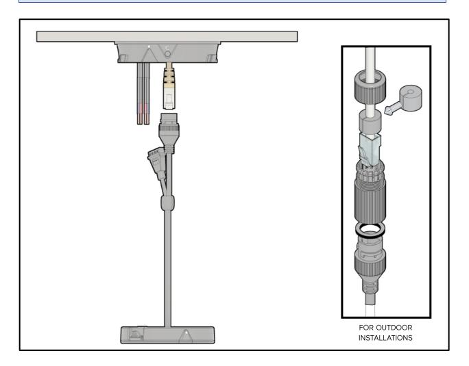
2. Connect the Alarm I/O as required.
