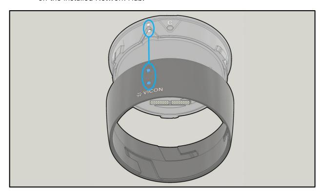
4. Twist the Solo Fixture to the right to lock it into place. The Vicon logo on the Solo Fixture is now aligned with the Base's centerline ("C").
