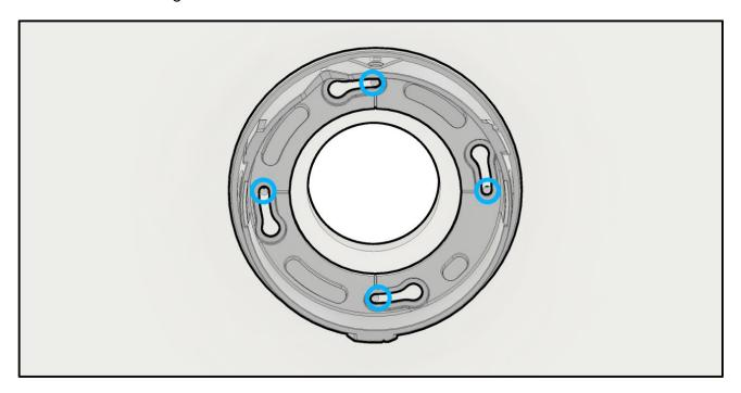
Reminder: The "C" on the Base indicates the centerline, which is the lens home position. For ceiling mount applications, C = front of the camera; for wall mount applications, the C should be facing the floor.
