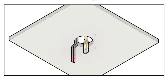
2. Once you've determined your centerline, use the Base to mark holes for the four mounting screws.
