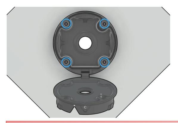
NOTE: The C indicates the centerline for the camera installation.
