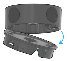
3. Remove the conduit plug from the cable access hole that will be used for conduit entry for this installation (there are 4x conduit plugs).
