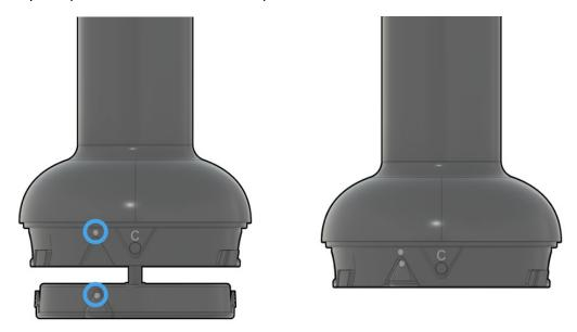
2. Align the two lock screws on the Solo Fixture with the double dot indicators on the installed Network Hub.
